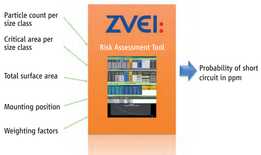
Fig. 95: Functional structure of risk assessment tool
