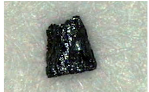
Fig. 33: Ferrite particle, identified as non-metallic (558 \mu\text{m} )
