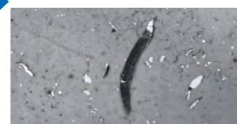
Metallic particle 1623 µm
