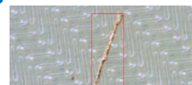
Metallic particle 421 \mu\text{m}
