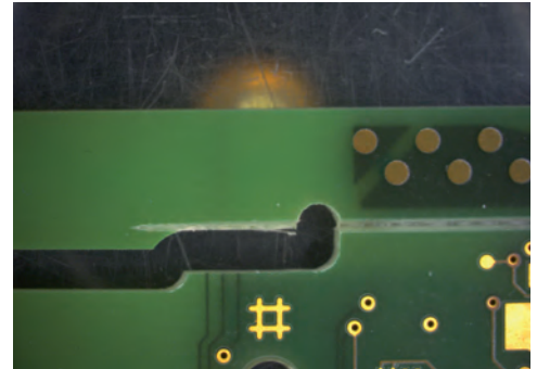
Fig. 58: V-scoring line on milling edge
