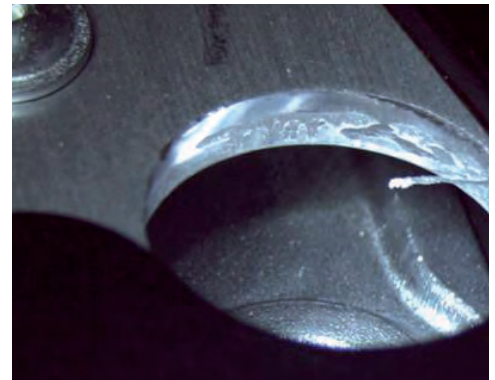
Fig. 69: Stamping residue loosened by pickling bath
