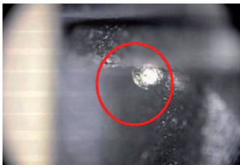
Fig. 33: Ferrite particle, identified as non-metallic (558 \mu\text{m} )
