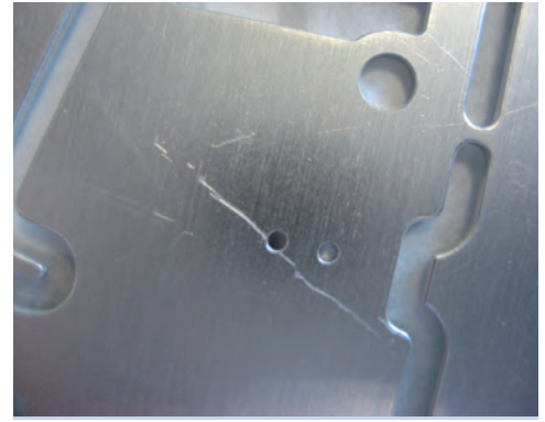
Fig. 67: Damaged metallic stiffener
