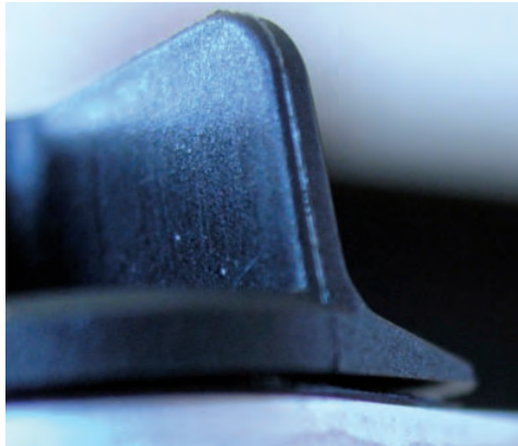
Fig.70: Plastic element with burr
