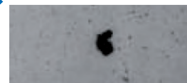
Non-metallic particle 261 \mu\text{m}
