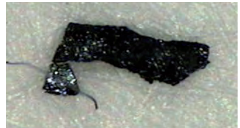
Fig. 34: Non-metallic particle, probably burr or plastic residue (217 \mu\text{m} )
