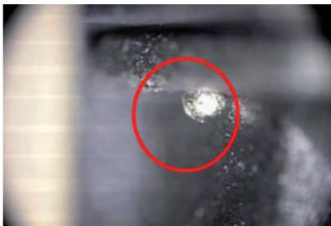
These solder balls can also be found squeezed flat on housings as carry-over particles. Since tin is soft, small balls on table tops or between tools are pressed flat and easily adhere to rough surfaces.
