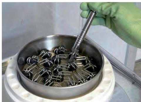
The components are then removed and the empty component holder with container is rinsed as part of the extraction process.
