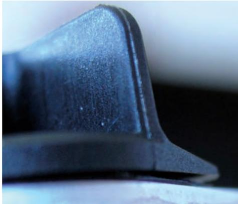
Fig. 71: Particles on externally supplied plastic elements
