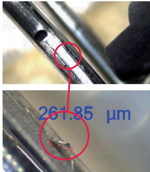
**Fig. 27: Enlarged photo depicting particle length measurement**
