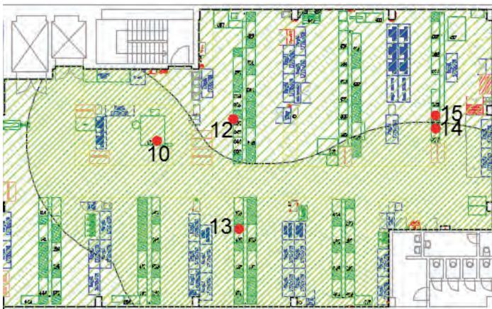
This is due to the chosen locations of the particle traps. Particle traps 2, 6, 7, 10, 12, 13, 14 and 15 were placed away from the manufacturing processes to collect particles from the ambient air environment<sup>1</sup>. Particle traps 1 and 3 were placed within the processing area and have recorded the process environment<sup>2</sup> in addition to the ambient air environment.
