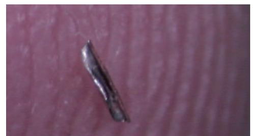
**Fig. 26: Particle (tin) adhering to a tinned copper wire D = 2.25 mm**
