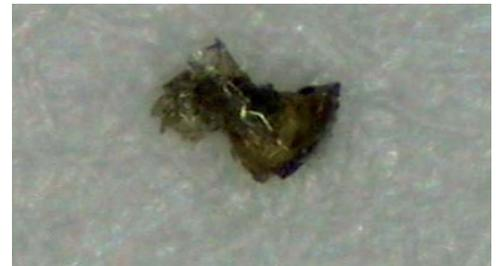
**Fig. 35: Non-metallic particle, probably pink polystyrene packaging material**
