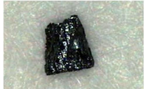
**Fig. 33: Ferrite particle, identified as non-metallic (558  $\mu\text{m}$ )**
