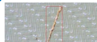
Fig. 52, 53: 12-pin connector with bridged contacts
