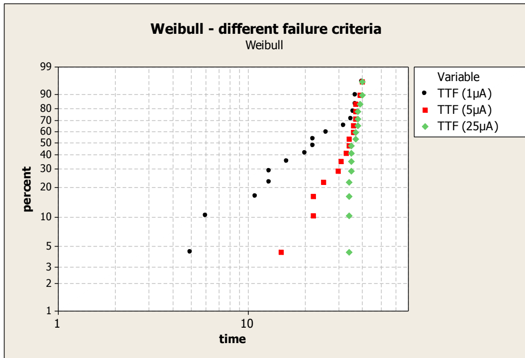
Figure 13: Weibull graph for different failure criteria (correspondent to Figure 5)
