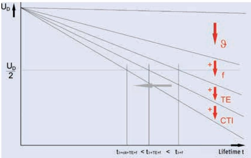
Reduction of the potential operating time by reduction of the breakdown voltage due to temperature, frequency, partial discharge (electrical stress) and environmental conditions (Source: CMC)
