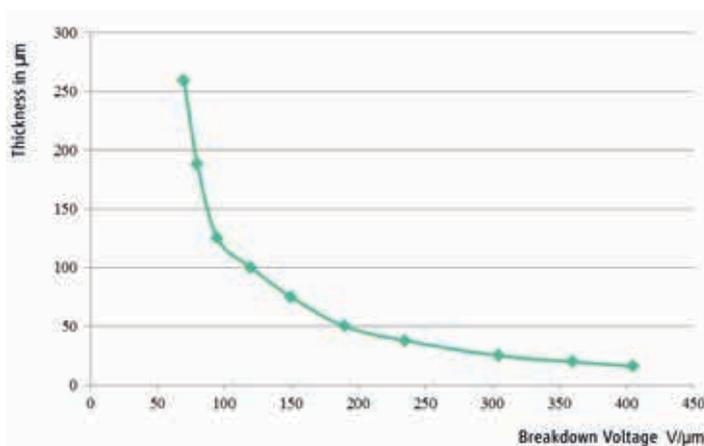
Breakdown voltage vs. material thickness of polyester foil (Bsp.: PET, Source: CMC)
