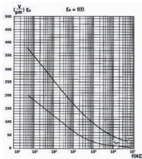
Dependency of the breakdown voltage vs. frequency
