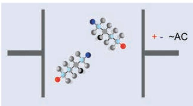
Repolarization losses in insulation materials (Source:CMC)
