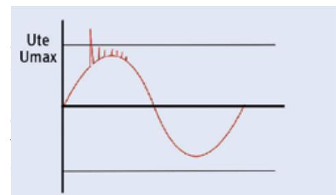
Triggered PD even below PD inception voltage operation conditions (Source: CMC)
