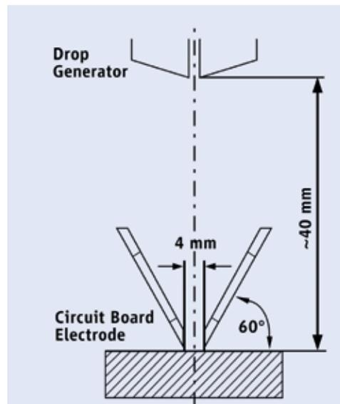
Measuring the CTI value on insulating materials (Source: UL 746)
