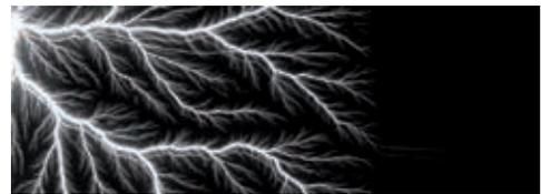
Formation of a conductive path on or in insulation materials
