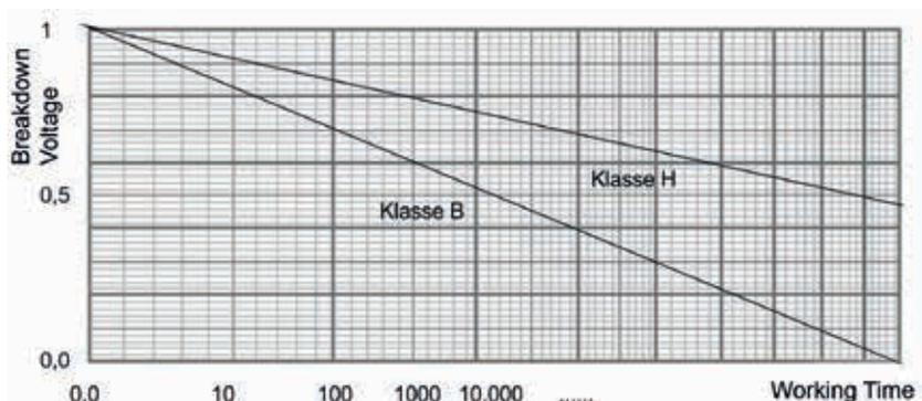
Half the breakdown voltage according to UL 746 at 130 °C (Quelle: CMC)
