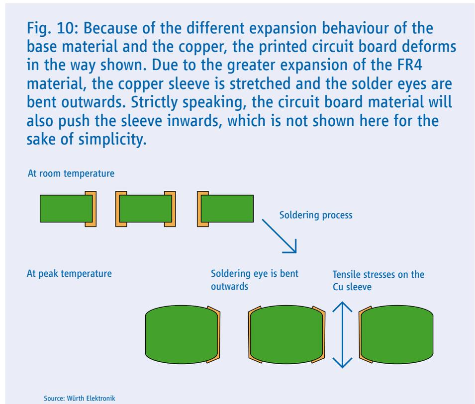
In the worst case, these stresses in the sleeve can lead to cracking and thus to electrical interruption, i.e. a failure.
