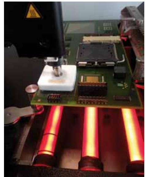
Programme sequence: Change of position of hot gas nozzle and vacuum pipette and subsequent lifting by means of vacuum-assisted pipette.
