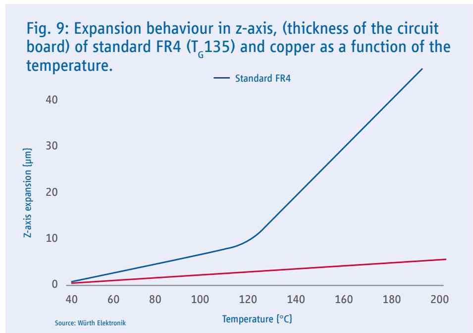
This difference in the expansion coefficient causes the plated through holes to be pulled apart at high temperatures in the circuit board and the soldering pad to be pressed outwards, as shown schematically in the following figure.
