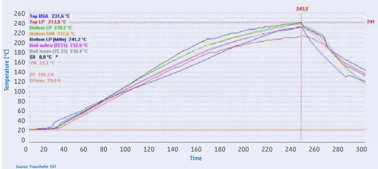
Figure 23 shows the temperature profile of the rework profile and Table 8 shows the determined soldering parameters.
