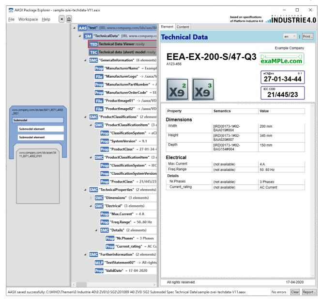
Figure 1 Screen shot of the AASX Package Explorer with Submodel "TechnicalData" of an example asset<sup>1</sup>, featuring multiple technical properties and visualization of the Submodel information via a specific plug-in "Technical Data Viewer"
