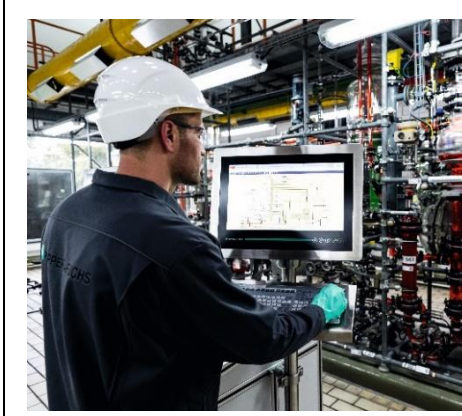
Fig. 22: Human Machine Interface intended for use in environments as defined in 2014/34/EU (ATEX)
